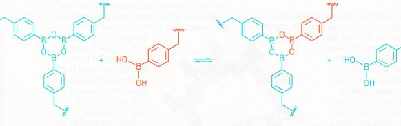
A thermoset polymer with boron-oxygen bonds has the ability to be reshaped and recycled, thanks to this chemical transformation.
