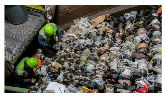
Workers sorting recyclables at a material recovery facility frequently struggle with plastic bag contamination. In this photo, bags can be seen tangling a star-wheel sorting system, preventing the proper separation of various materials.
