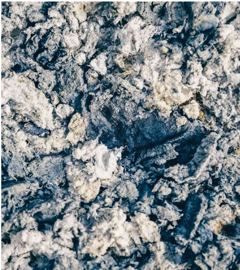
Renewcell creates a dissolving pulp from waste cotton that forms the basis for new cellulosic fibers.
