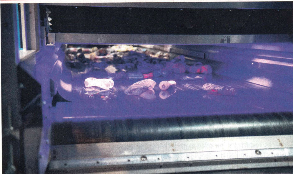
Left: A prototype sorting unit tested by the smart-packaging initiative HolyGrail 2.0 could improve the separation of plastic waste.
