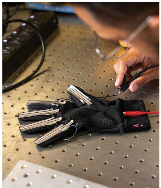
This reusable glove is made with a material that keeps the wearer's skin safely under 40 °C while the outer surface heats up to 100 °C for a few seconds when electric current passes through it.
