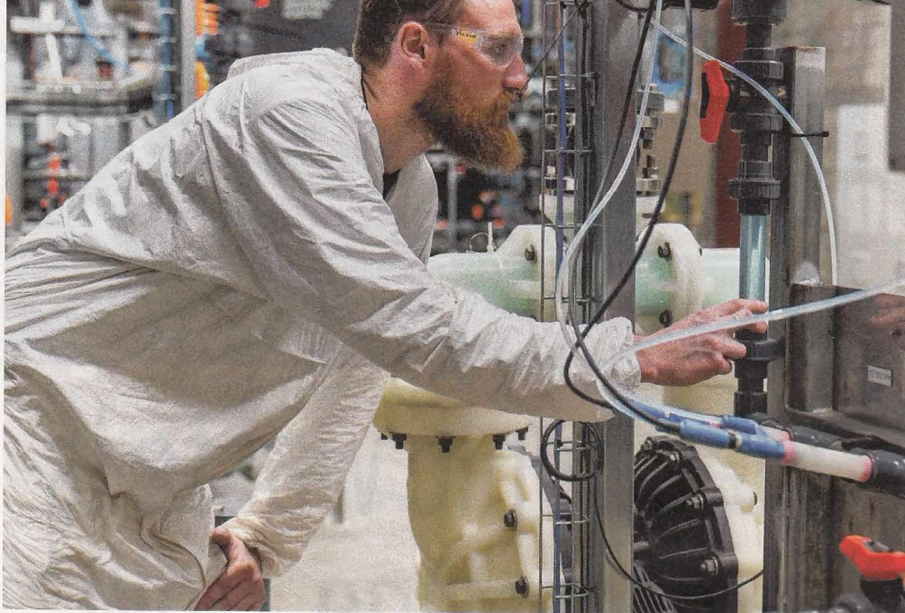
A worker at start-up Mint Innovation’s new commercial e-waste recycling facility in Sydney monitors the reactor carrying bacteria that extract gold from ground printed circuit boards.
